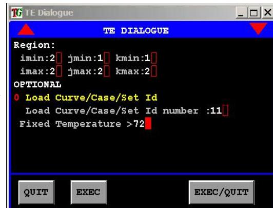
Use the TE option of the **CONDITION** command to view the nodal fixed temperatures in the merge phase.
