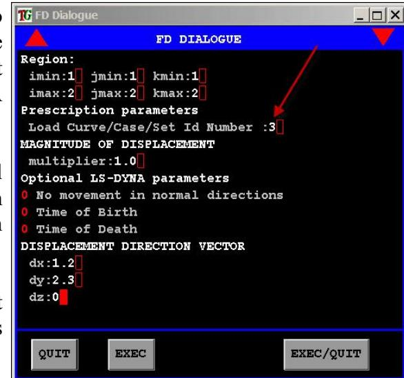
The FD command can also be found in the merge phase. Different methods are available in choosing the nodes to be displaced, including the need to create of a node set.
