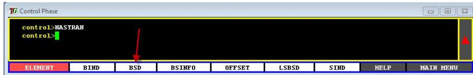
Use the BSD command, within the Element menu, to define the cross sectional properties of 1D elements.
