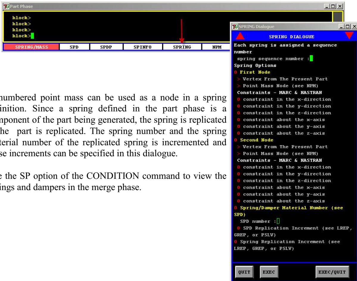
A numbered point mass can be used as a node in a spring definition. Since a spring defined in the part phase is a component of the part being generated, the spring is replicated if the part is replicated. The spring number and the spring material number of the replicated spring is incremented and these increments can be specified in this dialogue.
