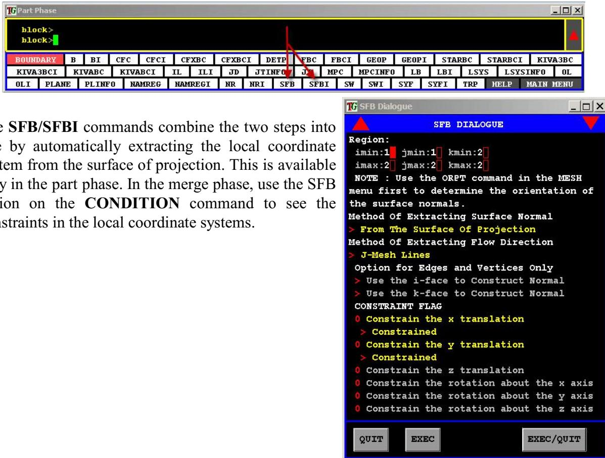
The **SFB/SFBI** commands combine the two steps into one by automatically extracting the local coordinate system from the surface of projection. This is available only in the part phase. In the merge phase, use the SFB option on the **CONDITION** command to see the constraints in the local coordinate systems.
