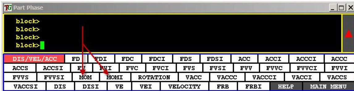
On the right is the dialogue for the MOM command in the part phase. The dialogue for the MOMI is similar. If the prescription is about a general axis, this command will be needed three times, one for a component about each axis.
