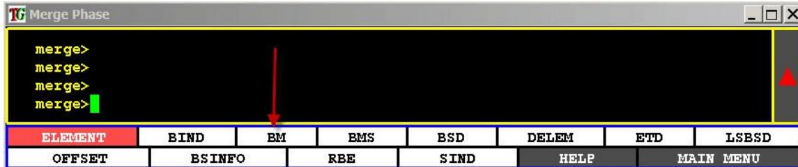
The BM command in the merge phase, used to create 1D elements, also has the options to specify 1D element properties, identical to the beam commands in the part phase.
