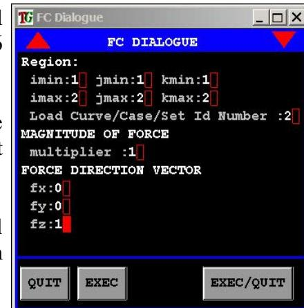
The FC command can also be found in the merge phase. Different methods are available in choosing the nodes for nodal forces, including the creation of a node set.
