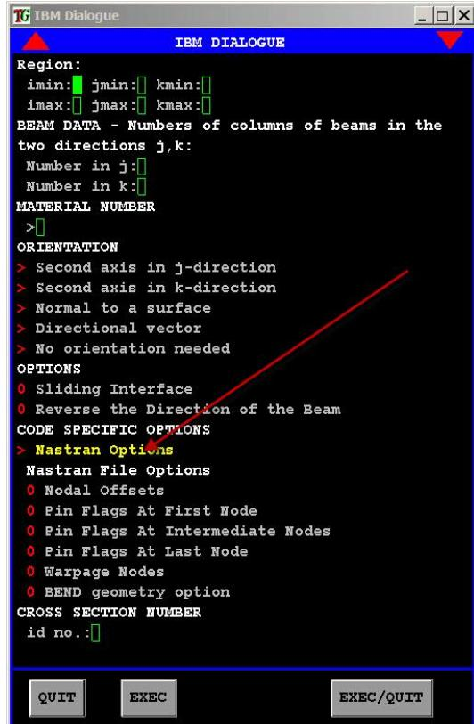
The beam commands in the part phase can assign some properties to the 1D elements being generated. In particular, if the 1D element is a beam, then nodal offsets, pin flags, and warpage points can be specified. If the 1D element is a bend, then the geometry option can be selected. These properties are only assigned to the 1D elements being generated by this instance of the beam command.
