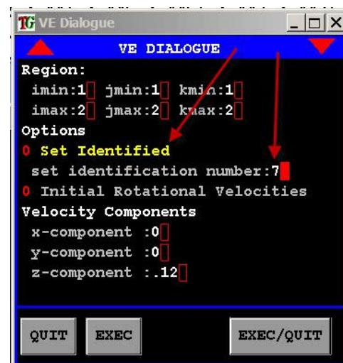
To specify rotational initial conditions, click on “Initial Rotational Velocities (Displacements)” so that it is yellow (left). The ve and dis commands are available in the merge phase using nodal sets instead of regions.
