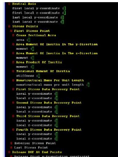
Notice, for example, the keyword **BNA1** in square brackets in the picture in the upper left, which selects tapered beam properties. Also, the stress points parameters (see the picture of the menu cut-out on the above right), which are numerous, are hidden until one selects one of the stress point options. All of the keywords, their meaning, and the associated parameters for the **BSD** command are listed below.
