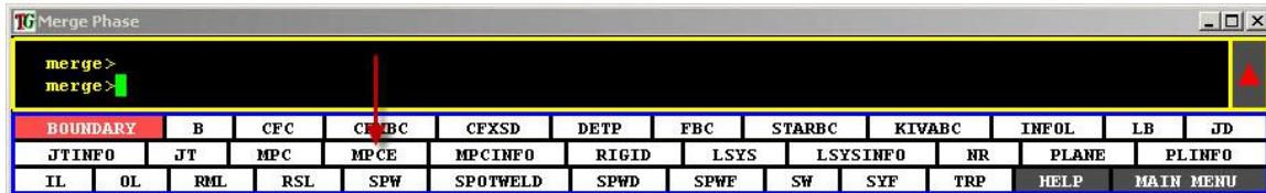
The first method is to use the **MPCE** command in the merge phase. This command is the most complicated because it supports many features. The set identification of the MPC and both coefficient and degree of freedom can be chosen for each node. This method requires either a node set or a list of nodes to form the MPC.
