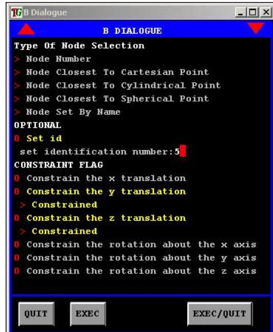
will create a SPC1 card in the NASTRAN® output file instead of incorporating the constraint in the GRID card. These constraints will only be active if the “SPC = 23” appears in a subcase.
