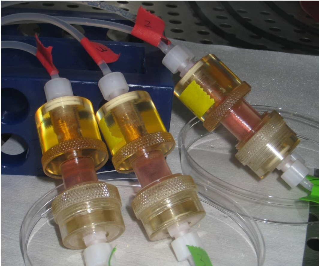
Figure 2.4. Flow chambers housing hASC-seeded scaffolds during pulsatile fluid flow stimulation. Fluid flow occurred in an upward direction from green to red labels.
