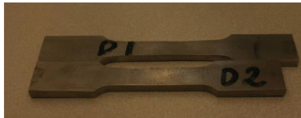
Figure 5.4. Test specimens D1 and D2. The upper D1 after testing and the lower D2 before testing
