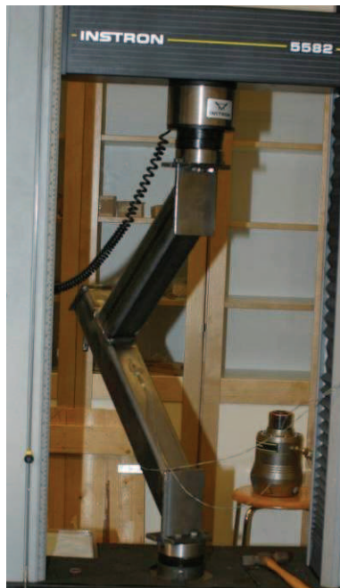
Figure 4.5. Component in test machine before loading
