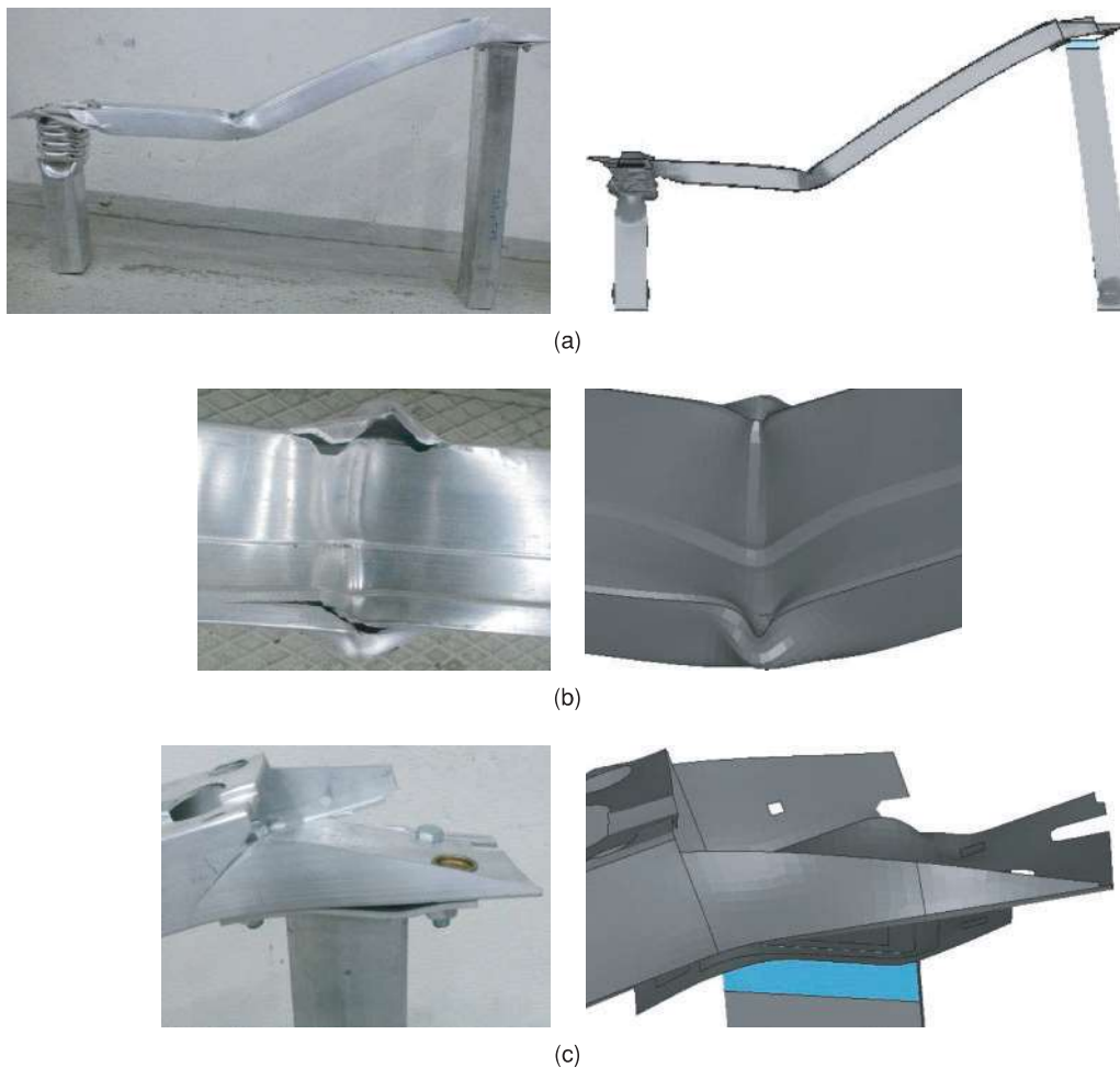
Figure 13 Comparison of permanent deformation shapes of test specimen A1 [4] and that obtained from simulation with MAT-41(CFS*).
