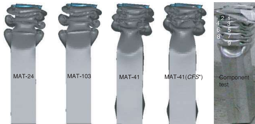
Figure 8 Development of lobes in the impacted longitudinal in simulations and test.
