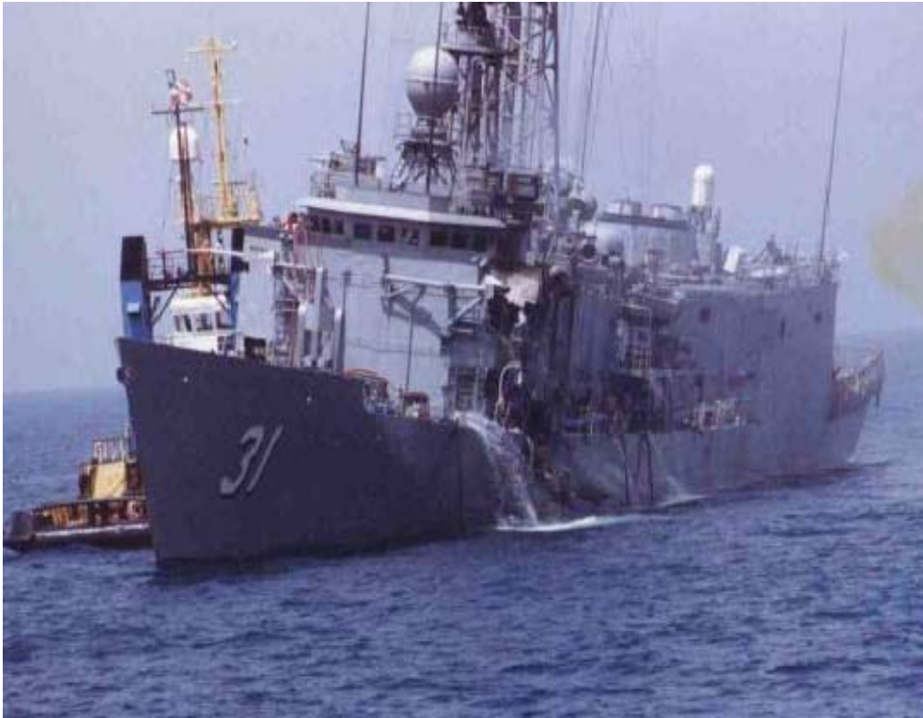
Figure 16 - USS Stark Damaged by 2 Exocet Missiles [32]
