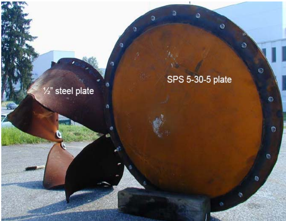
Figure 115 - US Navy Blast Test Results for Steel and SPS Plates [28]
