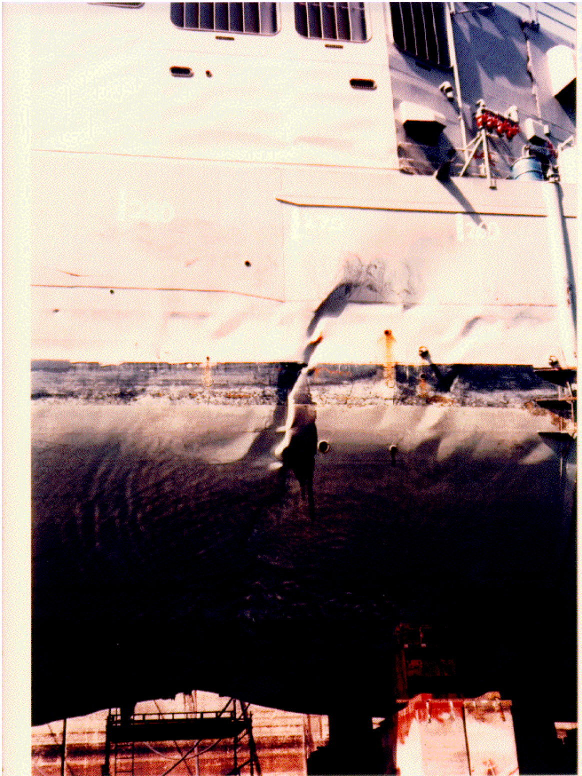
Figure 7 - USS Samuel B. Roberts – Close-up of Contact Mine Damage [34]
