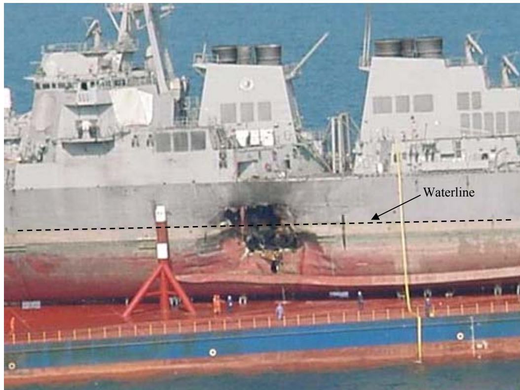
Figure 12 - USS Cole – AIREX and UNDEX Contact Explosion Showing Damage Above and Below the Waterline [32]
