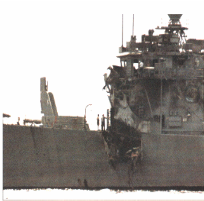
Figure 14 - USS Stark – Penetrating Internal Air Explosion [32]
