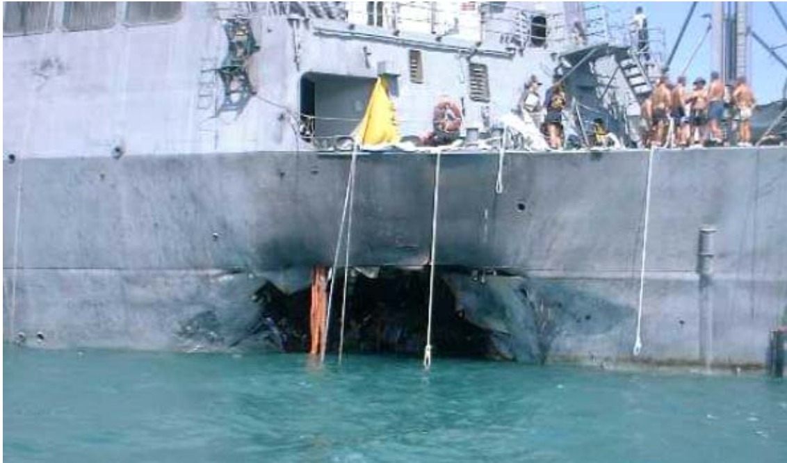
Figure 11 - USS Cole – AIREX and UNDEX Contact Explosion [32]
