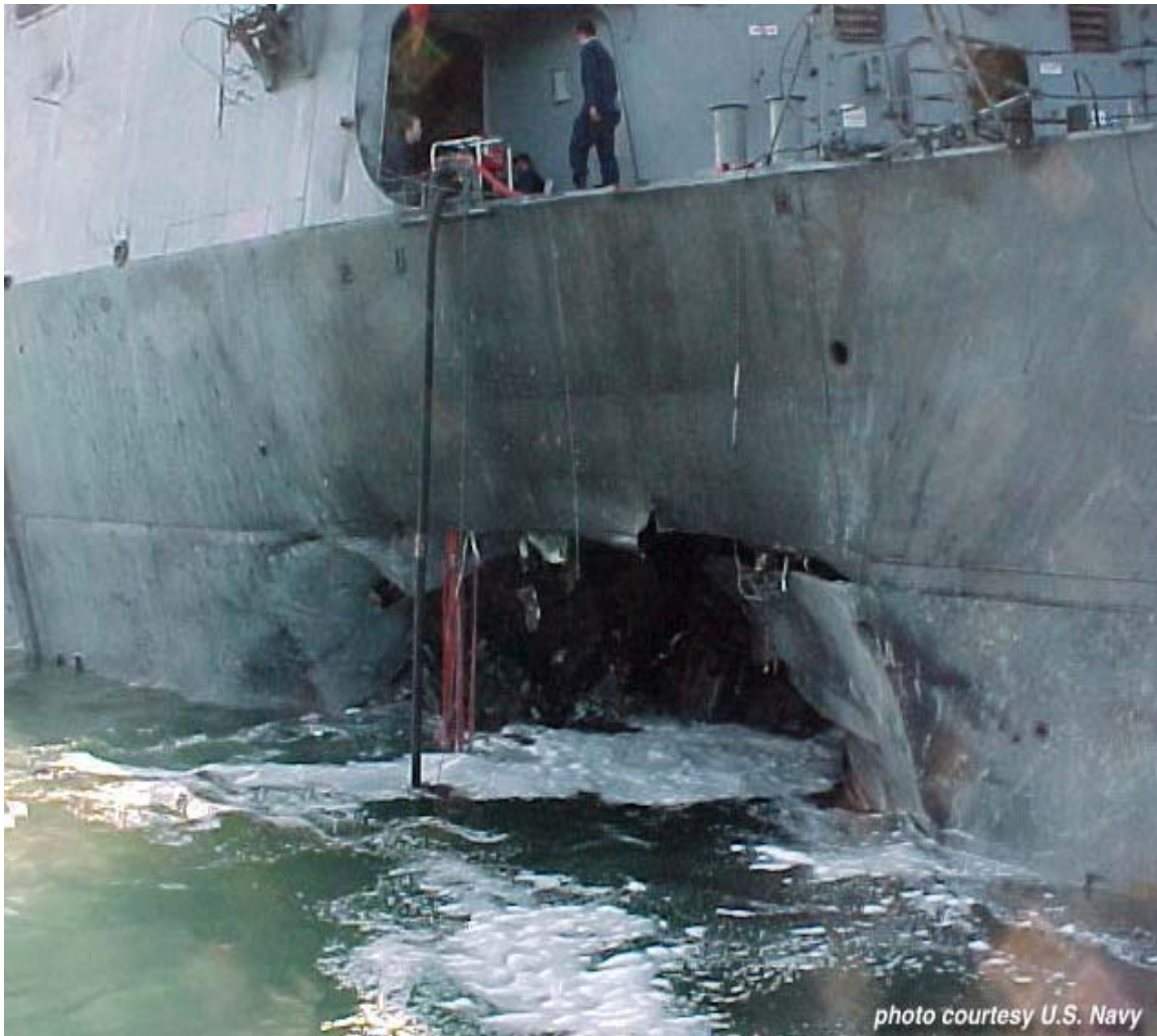
Figure 13 - USS Cole AIREX and UNDEX Contact Explosion [32]
