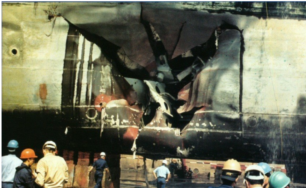
Figure 5 - USS Tripoli – Contact Mine [3]
