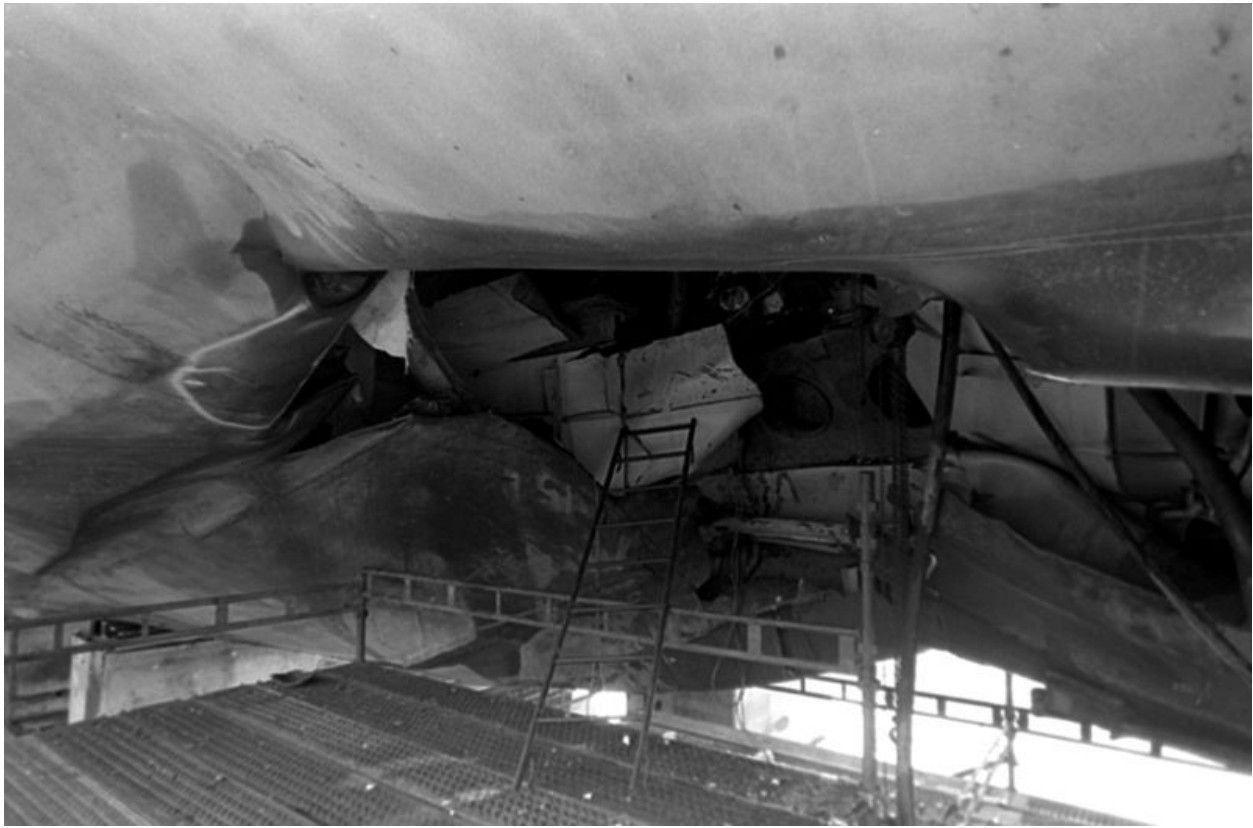
Figure 6 - USS Samuel B. Roberts – Contact Mine Damage Under Keel [35]
