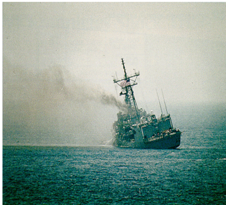
Figure 15 - USS Stark Shown with a List Due to Compartment Flooding [32]
