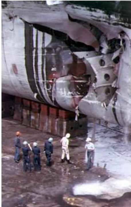
Figure 4 - USS Tripoli – Contact Mine [34]
