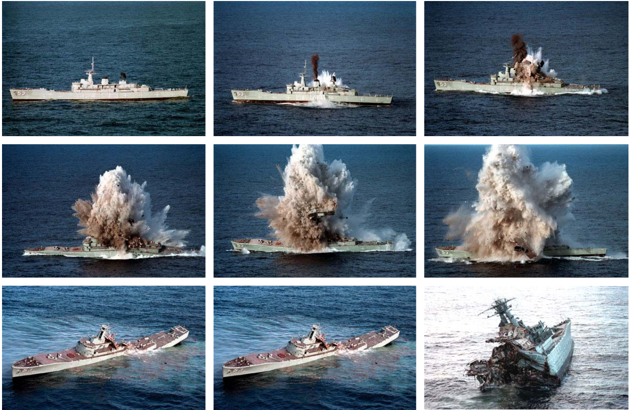
Figure 10 - Australian Navy MK 46 Torpedo Test (Under Keel) [32]
