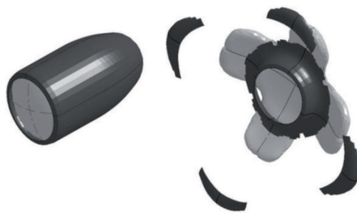
Fig. 5. Projectile deformation in the final stage – numerical result
