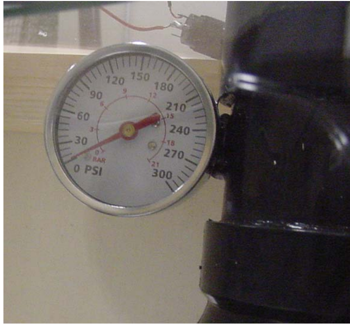
Figure 9: Air pressure sensor connected to the storage chamber.
