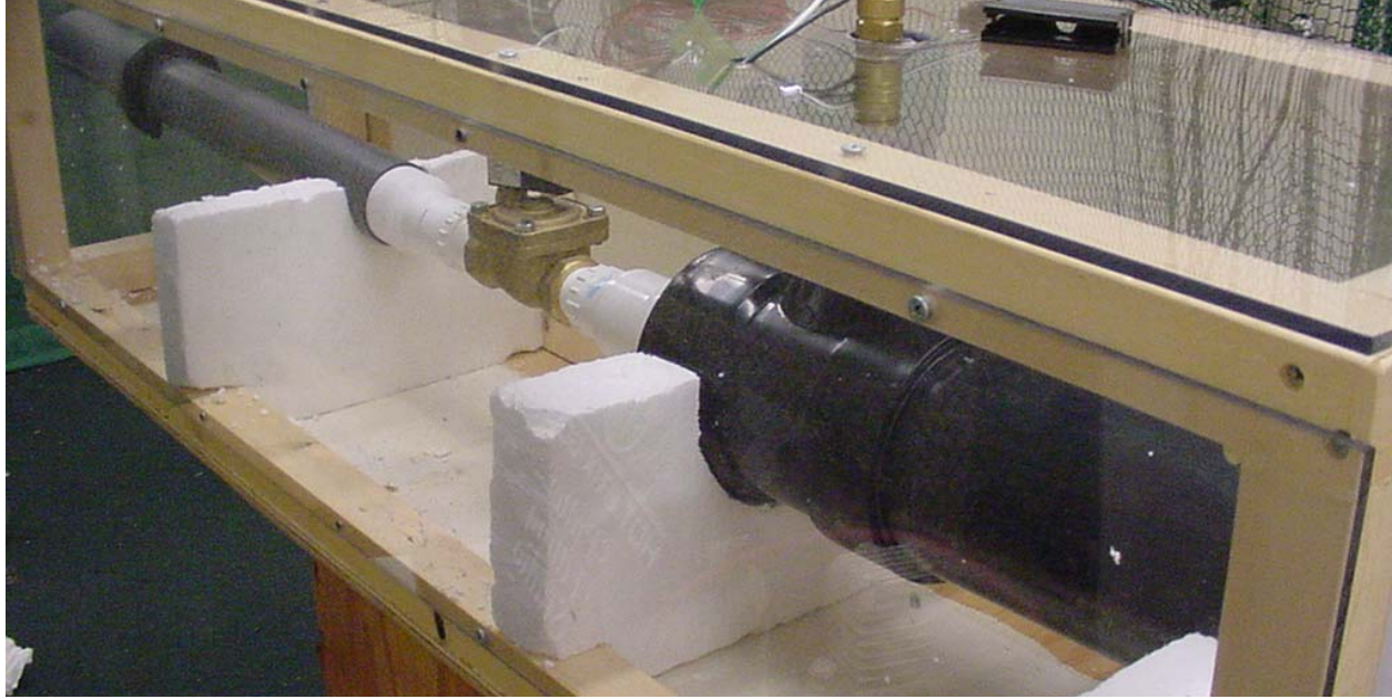
Figure 11: Air cannon placed on test stand behind 1/2" polycarbonate.
