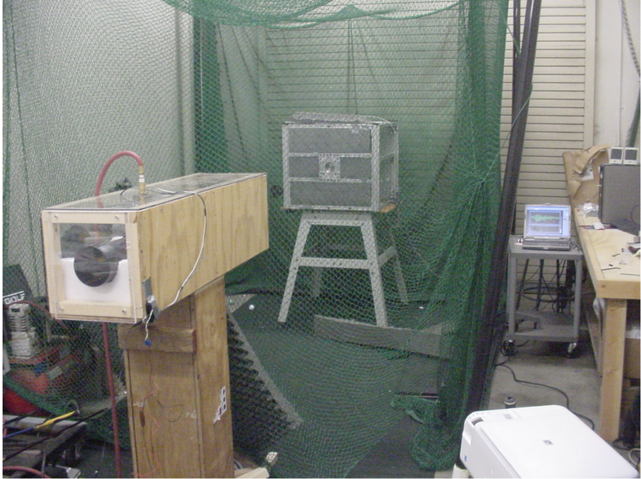
Figure 7: Experimental setup to determine the sound output of the titanium plate. Shown is the air cannon, plate support structure and data acquisition system.
