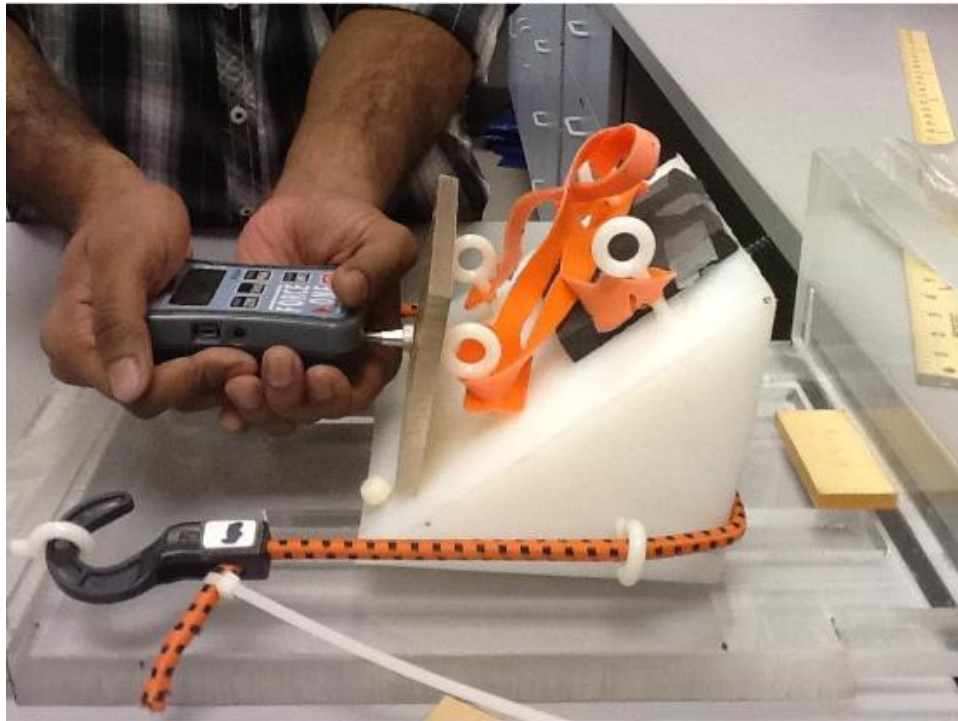
Figure 3.1: The loading frame used during the MRI scan procedure.
