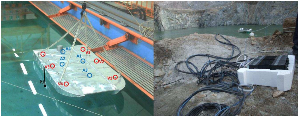
Figure 4.14 Locations of sensors and analyzer.
