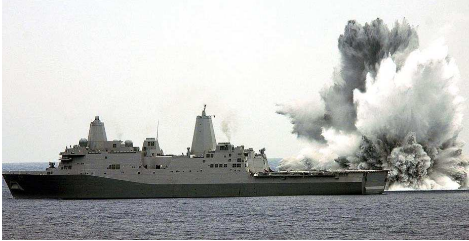
Figure 6.1 Large-scale ship shock test 2008 (USS, underwater explosion).
