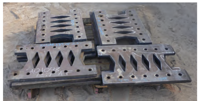
Fig. 8. (a) Elevation drawing and (b) photograph of strongback frame for the Tesla facility; (c) Krawinkler fuses (images courtesy of Gregory P. Luth & Associates).
