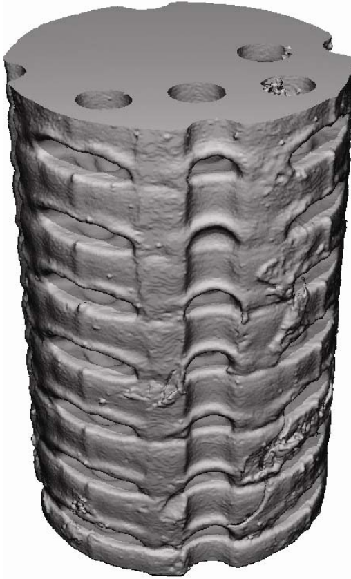
Figure 6.2: Micro-CT image of a scaffold fabricated using stereolithography (rapid-prototyping). Image courtesy of Professor David Dean, Case Western Reserve University.
