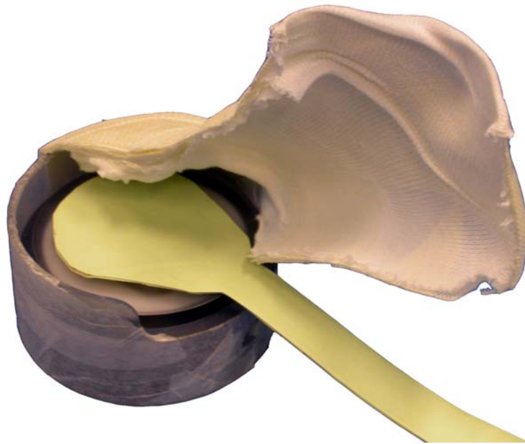
Figure 2.3. The loading device was attached to the subjects' feet using fiber-glass casting material. Here, the medial half of the cast has been removed to show the device beneath and the Pliance® pressure sensitive array fixed to the top of the loading plate.
