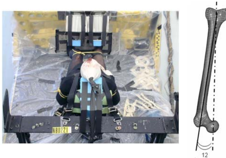
Figure 5.41. Initial adduction angle in cadaver test (left) and anatomical adduction angle for the femur bone in its natural position (right). (Rupp, 2002)
