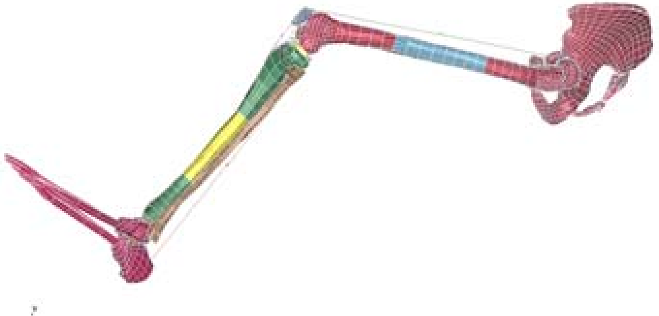
Figure 4.1. The LLNL KTH model of the lower extremity. (Perfect, 1997)
