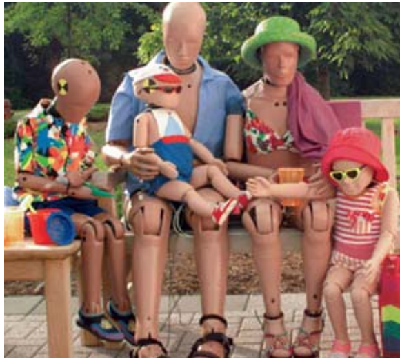
Figure 2.11. ATDs of different sizes to be used in car crash tests. (edmunds.com, 2007)
