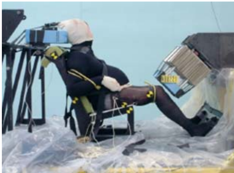
Figure 2.10. Cadaver used for a sled test. (UMTRI, 2002)
