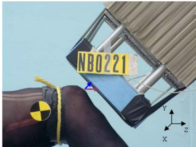
Figure 5.29. Knee bolster made of floatation foam material used in the sled cadaver test. (Rupp, 2002)
