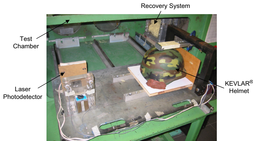
Fig. 1. The set-up for the ballistic impact test of a KEVLAR ® helmet.
